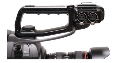
The handle can take two audio inputs by using XLR cable.
